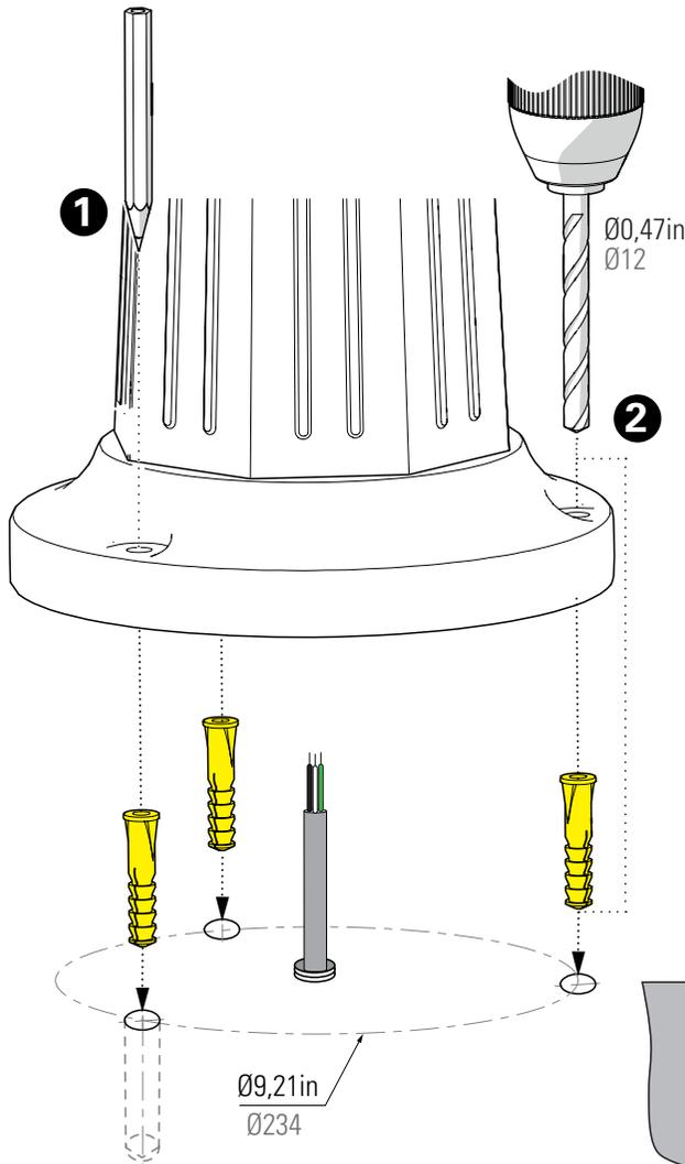
**2** Mount the head assembly on the mast
